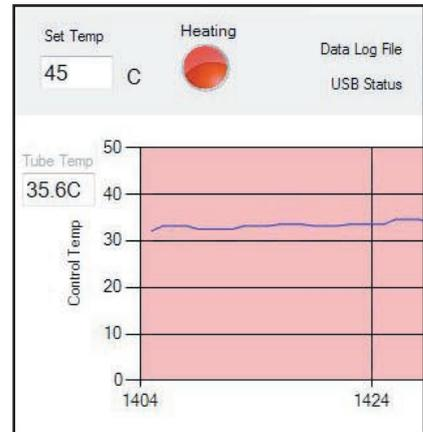
Rodent body temperature can be continuously displayed and recorded via computer using Darvall's integrated software.
