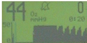
During expiration in animals with large chests, heart beats can force small puffs of gas up the trachea causing "bumps" in phase "C" of the ETCO<sub>2</sub> waveform.
